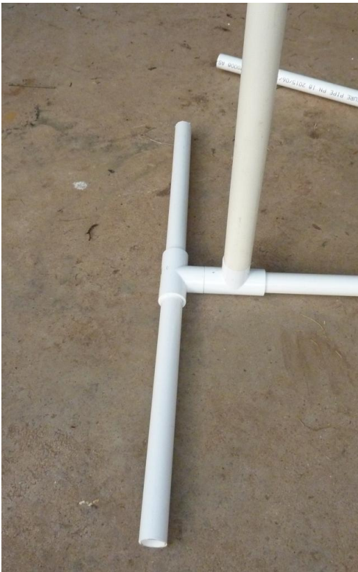
The base at both ends (2 T-joiners)
