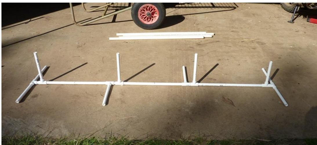
The base for the 3 X 4's. The larger diameter pipes fit over the uprights for easy removal
